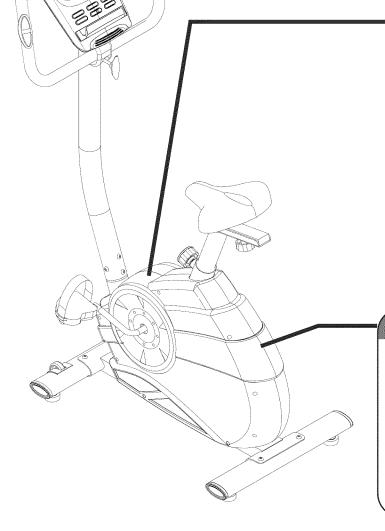
Lock the Front Stabilizer (31) and Rear Stabilizer (32) to the Main Frame (29) by using the wrench (87), Hex Bolt (30) and Washer (26).
