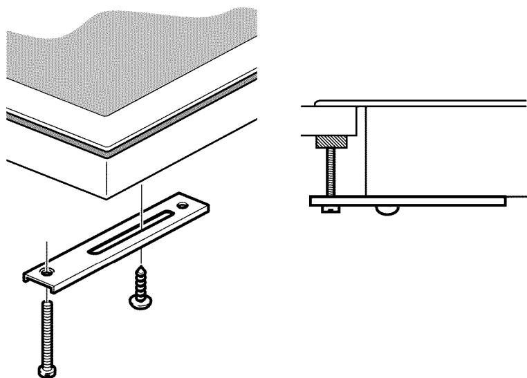
The cooktop should be secured to the countertop using the hold-down brackets provided.
