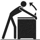
To check if the anti-tip bracket is installed properly, use both arms to grasp the rear edge of the appliance back. Carefully attempt to tilt appliance forward. When properly installed, the appliance should not tilt forward.
