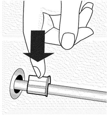
3. Slide the shelf grommet into the grommet already in the freezer wall until it is flush.
