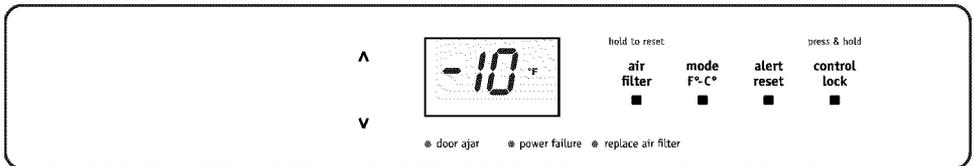
To adjust the temperature setting, press the UP (▲) key for warmer temperature and DOWN (▼) key for colder temperature on the control panel. Allow several hours for the temperature to stabilize between adjustments. The unit can be adjusted between -10°F (-23°C) and 10°F (-12°C). By pressing the TEMP MODE key, the temperature display will toggle between °F and °C.
