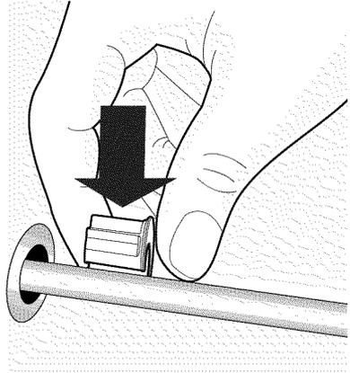
2. Push the shelf grommet onto the wire until it snaps in place.
