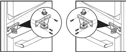
Once both doors are in place, ensure they are aligned with each other and level (Please see the "Installation" section for more details), and replace the top hinge cover.
