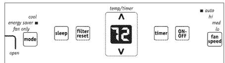
Note: The unit will run in energy saver mode when used for the first time. In this mode, the fan will continue to run for 1 minute after the compressor shuts off. The fan then cycles on for 20 seconds at 10 minute intervals until the room temperature is above the set temperature, at which time the compressor turns back on.
