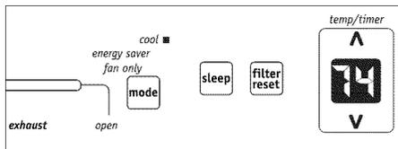
Note: In this mode, the fan remains on all the time with the compressor cycling on and off when room temperature is reached.
