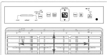
The 4-Way air directional louvers allow you to direct the air flow Up or Down and Left or Right throughout the room as needed.
