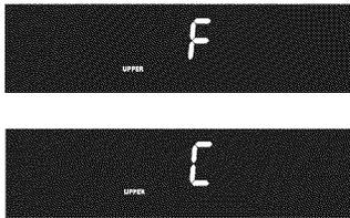
Figure 17: Control showing Fahrenheit (top) or Celsius (bottom)
