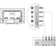
connect a HDMI device, such as a DVD player, please Connect the HDMI 1/ARC, 2/DVI jack on the side of  $\overline{\text{TV}}$  to the output jacks of device via HDMI cable.
