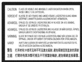
This label is located on the laser protective housing inside the enclosure.
