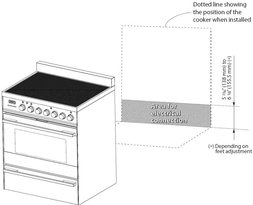
Grounded outlet: should be located from the left to the right side of the range; from 5" 7/16 (138 mm) to 6" 1/8 (155.5 mm) [depending on feet regulation] from the floor.
