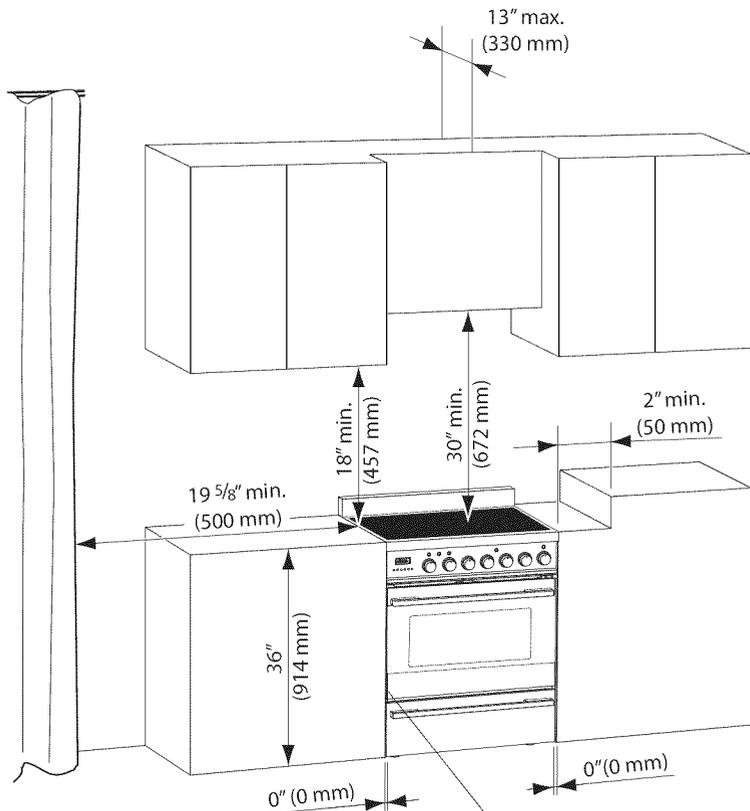
The range CANNOT be installed directly adjacent to sidewalls, tall cabinets, tall appliances, or other side vertical surfaces above 36" (914 mm) high.
