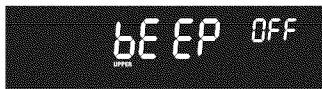
Figure 14: Control in bEEP OFF setting allows for silent operation of oven controls
