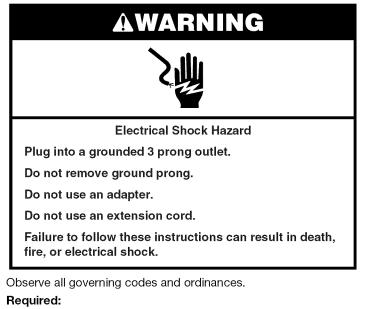
A 120 volt, 60 Hz, AC only, 15- or 20-amp electrical supply with a fuse or circuit breaker.
