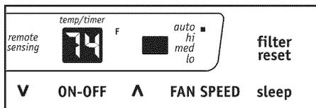
Note: Fan starts at High Speed and adjusts to a slower speeds the room temperature dictates. For example, if the room doesn't get too warm, it will stay at the slowest speed. If the room temperature rises quickly, such as a door being opened, it will automatically go to the highest speed. The fan speeds will re-adjust back to the slowest speed as the room returns to the original set temperature. Press either the fan slower or fan faster button to adjust the fan speed manually.
