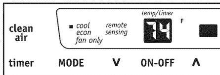
Note: In this mode, the fan remains on all the time with the compressor cycling on and off when room temperature is reached.
