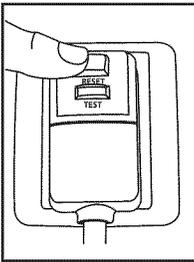
The power supply cord contains a current device that senses damage to the power cord. To test your power supply cord do the following:
