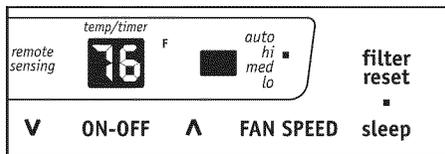
Note: In this mode the selected temperature will increase by 2 °F 30 minutes after the mode is selected. The temperature will then increase by another 2 °F after an additional 30 minutes. This new temperature will be maintained for 7 hours before it returns to the originally selected temperature. This ends the "Sleep" mode and the unit will continue to operate as originally programmed. The "Sleep" mode program can be cancelled at any time during operation by again pressing the "Sleep" button.
