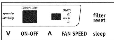
Note: If the unit is turned off in heat mode (if applicable) or fan only mode, it will return to the same setting when it is turned on again. When the unit is turned off in cool or energy saver(econ) mode, it will run in energy saver(econ) mode when it is turned on again, but the setting of temperature and fan speed will remain.
