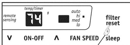
Note: This feature is a reminder to clean the Air Filter (See Care and Cleaning) for more efficient operation. The LED (light) will illuminate after 250 hours of operation. To reset after cleaning the filter, press the "Filter Reset" button and the light will go off.
