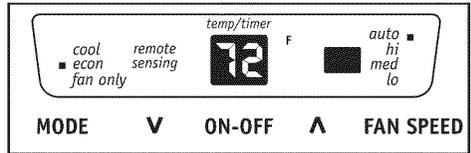
Note: The unit will run in energy saver(econ) mode when used for the first time. In this mode, the fan will continue to run for 1 minute after the compressor shuts off. The fan then cycles on for 20 seconds at 10 minute intervals until the room temperature is above the set temperature, at which time the compressor turns back on.
