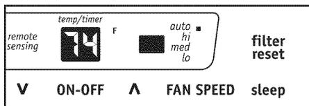
Note: Tap or hold either up ( ▲ ) or down ( ▼ ) button until the desired temperature is seen on the display. This temperature will be automatically maintained anywhere between 60 °F (16 °C) and 90 °F (32 °C) . If you want the display to read the actual room temperature. See "To Operate on Fan Only" section on Page 7.
