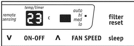
Note: The control is capable of displaying temperature in degrees Fahrenheit or degrees Celsius.
