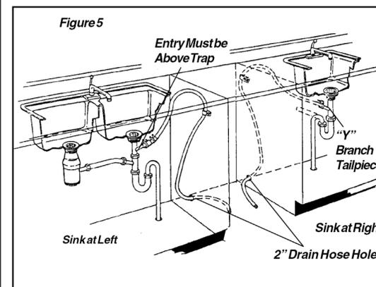
2. If you connect to a sink drain, entry will need to be above trap. A "Y" branch tailpiece and connector kit, not included, will make this method easier and includes all needed fittings and instructions. See Figure 5.
