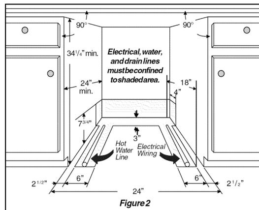
IMPORTANT: For proper operation and appearance of unit, cabinet opening should have dimensions as shown in Figure 2. If unit is to be placed in a corner, there must be at least a 2-inch side clearance to open door.
