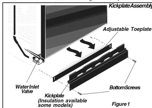
3. Locate water inlet valve behind kickplate on bottom left underside of unit. The valve has a  $\frac{3}{8}$ " NPT or  $\frac{3}{4}$ " hose thread fitting. Note: If using  $\frac{3}{4}$ " hose thread fitting skip steps 4 and 5.
