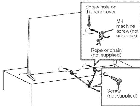
The length of the M4 machine screw differs depending on the rope or chain diameter. Please see below illustration.
