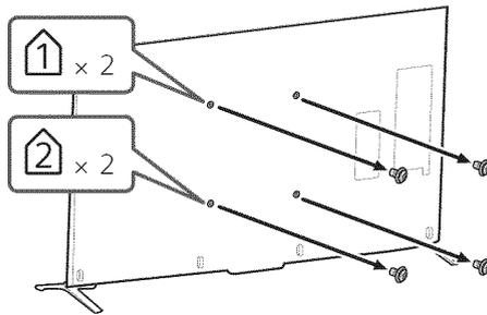
**2** Before installing the Wall-Mount Bracket, attach the Wall-Mount Attachment (supplied with the TV) to the rear of the TV (to make it parallel with the wall). (XBR-79/65/55X900B only)
