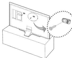
3. Connect the clamps fixed onto the TV and the clamps fixed onto the wall with a durable, heavy-duty string, and then tie the string tightly.
