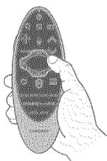
Press the directional buttons (up, down, left, and right) to move the focus, pointer, or cursor in the direction you want.
