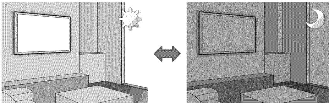
Eco Sensor measures the light in your room and optimizes the brightness of the TV automatically to reduce power consumption. This causes the TV to brighten and dim automatically. If you want to turn this off, go to **MENU > System > Eco Solution > Eco Sensor**.
