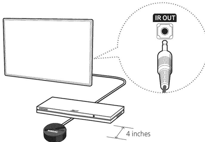
To begin the universal remote set up process, connect the IR extender cable (included) to the TV's IR output connector as shown in the diagram, and then position the transmitter end within 4 inches (10 cm) of the external device's remote control sensor, pointing in the direction of the sensor.
