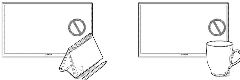
Do not block the sensor with any object. It can decrease picture brightness.
