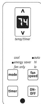
Note: Fan starts at High Speed and adjusts to a slower speed as the room temperature dictates. For example, if the room doesn't get too warm, it will stay at the slowest speed. If the room temperature rises quickly, such as a door being opened, it will automatically go to the highest speed. The fan speeds will re-adjust back to the slowest speed as the room returns to the original set temperature. Press either the fan slower or fan faster button to adjust the fan speed manually.
