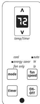
Note: The unit will run in energy saver mode when used for the first time. In this mode, the fan will continue to run for 1 minute after the compressor shuts off. The fan then cycles on for 20 seconds at 10 minute intervals until the room temperature is above the set temperature, at which time the compressor turns back on.
