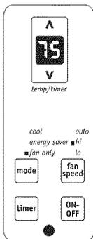
Note: Use this function only when cooling is not desired, such as for room air circulation or to exhaust stale air on some models. (Remember to open the vent during this function, but keep it closed during cooling for maximum cooling efficiency.) You can choose any fan speed you prefer. (Except "Auto Fan"). During this function, the display will show the actual room temperature, not the set temperature as in the cooling mode.
