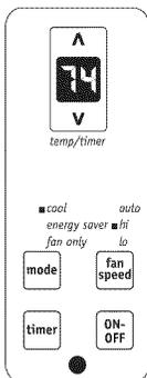
Note: In this mode, the fan remains on all the time with the compressor cycling on and off when room temperature is reached.
