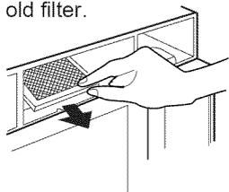
6. Slide a new charcoal filter into place and close the door. The filter should rest at the angle shown.
