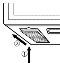
**NOTE:** Do not operate the hood without the filters in place.
