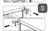
3. Remove the screws from the upper right hinge. Place the upper right hinge in a safe place in case you need to reverse the door in the future. Remove the plastic caps from the upper left hinge corner. Install the upper left hinge by fastening the screws through the left hinge to the cabinet. Insert the plastic caps to the upper right corner.
