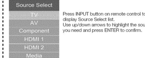
Press INPUT button on remote control to display Source Select list. Use up/down arrows to highlight the source you need and press ENTER to confirm.
