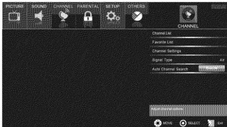
Use up/down to choose the function you need, press ENTER or right arrow to adjust or enter a sub-menu. The sub-menu image and explanation are shown below.
