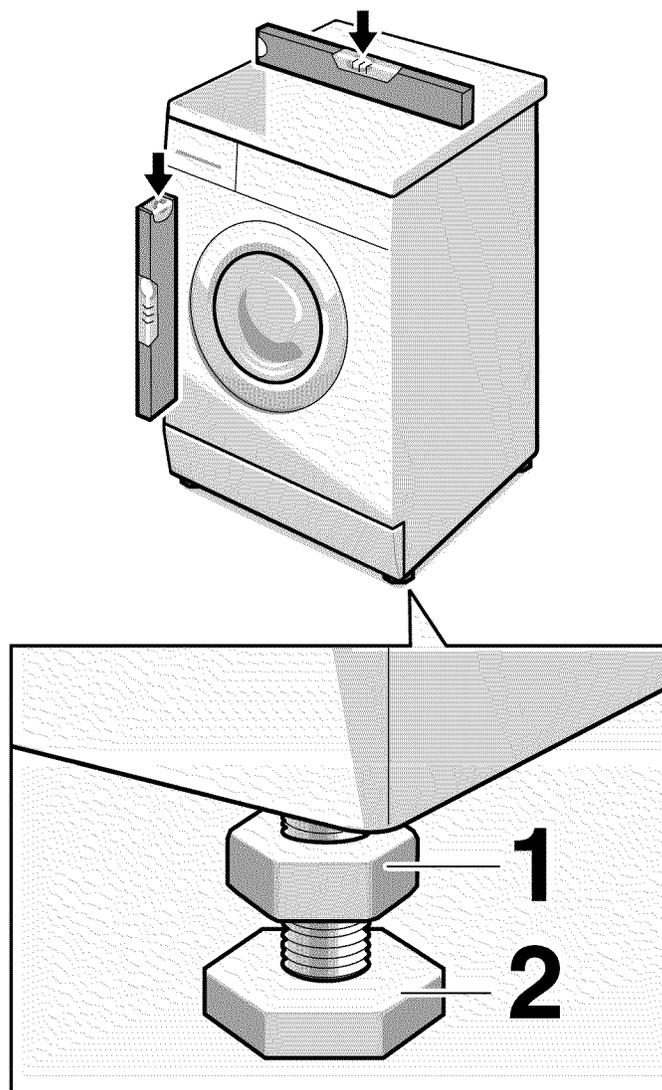
Level the washing machine with the assistance of the four adjustable feet and a spirit level:
