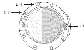
17. Install the DOOR on the 2 screws of BRACKET DOOR.
