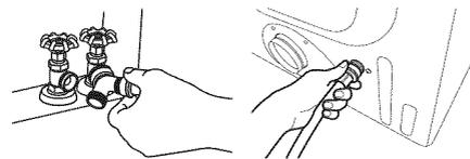
6. Using pliers, tighten the coupling with an additional two-thirds turn.
