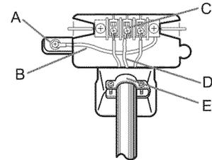
1. Loosen or remove the center terminal block screw.
