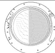
15. Assemble the COVER HANDLE and LEVER DOOR on the HOLDER GLASS.
