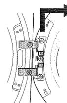
5. Remove the RING-E and PIN from the BRACKET DOOR.
