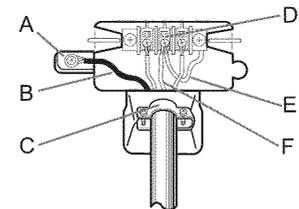
1. Remove the External ground connector screw.
