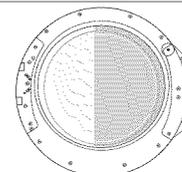
13. Rotate the HOLDER GLASS (BIG ROUNDED STEEL) 180°.
