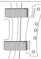
7. Remove the 4 screws (M4 2EA, M5 2EA), HOLDER LEVER, COVER HINGE, BRACKET LEVER from the left side of FRONT.
