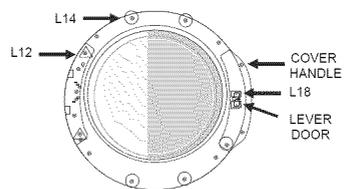
12. Remove the the 1 screw(L14).
