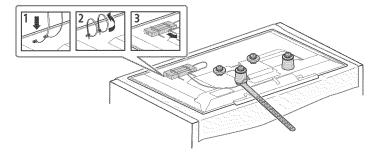
5  $\,$  Install the TV to the Base. Refer to "5" of Installation Guide and "Installing the TV to the Wall" of Operating Instructions supplied with the Wall-Mount Bracket.
