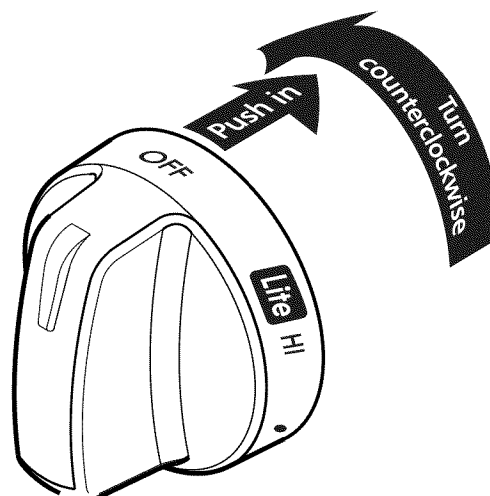
Figure 7: Correct way to set burners
