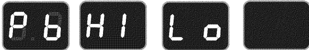
Figure 5: Range from Power Boost (Pb) to Hi setting to Lo and OFF (blank display)
