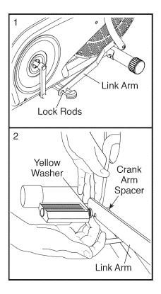
and downward slightly to make sure that they are fully seated on the crank arm spacers. CAUTION: Make sure that the link arms are fully seated on the crank arm spacers. If the link arms are not on the crank arm spacers, they may slip off during use, resulting in injury to the user.
