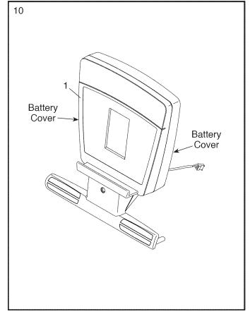
11. See the inset drawing. While a second person holds the Console (1) near the Upright (4), connect the wires on the Console to the Console Wire (5) and to the Ground Wire (15).
