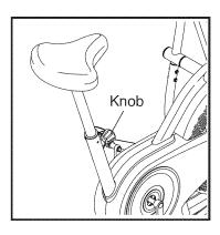
sure that the pin on the seat knob is engaged in one of the adjustment holes in the seat post. Then, tighten the seat knob.
