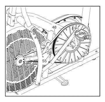
When the drive belt is correctly adjusted, reattach the left shield.
