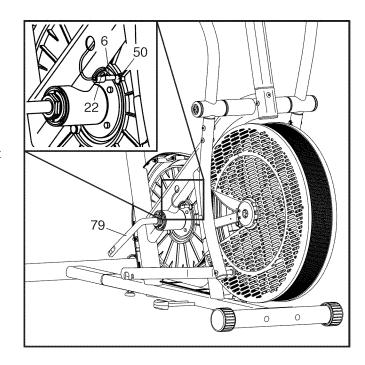
Loosen, but do not remove, the M4 x 15mm Tek Screw (22). Then, slide the Reed Switch (6) slightly closer to or away from the Magnet (50), and retighten the Screw. Turn the Right Crank Arm (79) for a moment.
