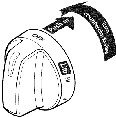
Figure 8: Correct way to set burners
