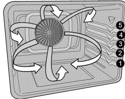
Figure 16: Air circulation in the convection function
