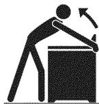
To check if the anti-tip bracket is installed properly, use both arms to grasp the rear edge of the
