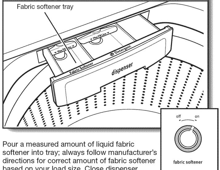
Pour a measured amount of liquid fabric softener into tray; always follow manufacturer's directions for correct amount of fabric softener based on your load size. Close dispenser drawer, then select Fabric Softener option. Fabric Softener is added during rinse.
