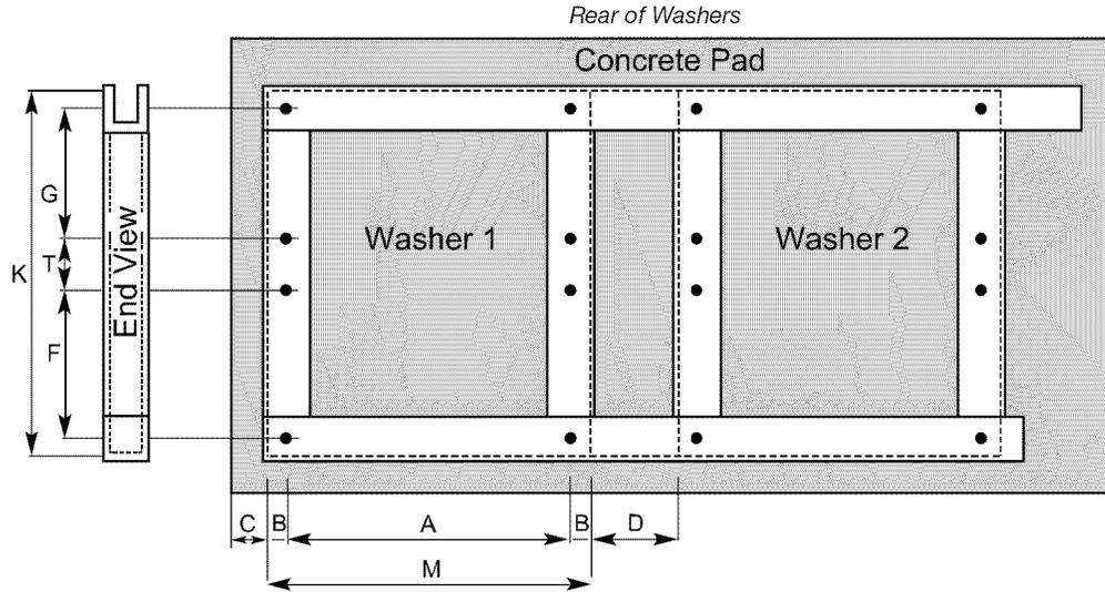
Dimension chart for foundation base, anchor bolt placement, and elevated concrete pad
