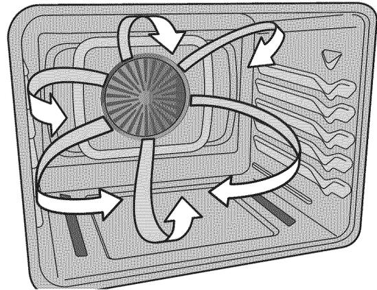
Figure 12: Air circulation in the convection function
