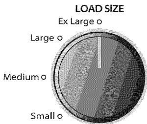
Select the load size setting most suitable for your load. Small will add a low amount of water for smaller loads and Ex Large will add the most amount of water for large or bulky loads. Items need to move freely.
