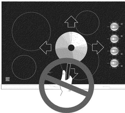
Sliding aluminum or copper clad bottom pans on the cooktop can cause metal markings on the cooktop surface. These marks should be removed **immediately** after the cooktop has cooled using the cooktop cleaning cream. Metal marks can become permanent if not removed prior to future use.
