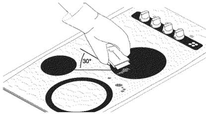
If soils remain, carefully scrape them with a metal razor blade scraper, holding scraper at a 30 degree angle to the surface. Remove loosened soils, then apply a few drops of cleaning cream and buff surface clean.
