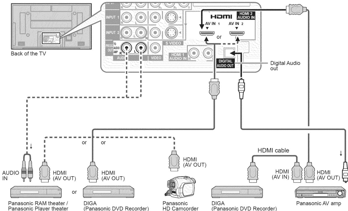
● One AV amp and one DIGA recorder can be operated with this unit.
