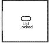
If you need to open the lid, press START/Pause/Unlock Lid. The lid will unlock once the washer movement has stopped. This may take several minutes if the load was spinning at high speed. Press START/Pause/Unlock Lid again to resume the cycle.
