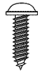
4 Phillips head screws to secure the transition to the hood outlet on the top
