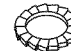
1 safety screw and lock washer, to secure the blower: (screw is marked with red or blue paint)
