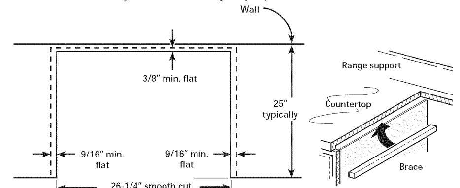
Countertop thickness 1-1/2" min. is required to support the product. Countertop width 1-1/2" min. is required to properly support the 3/4" anti-tip screw.
