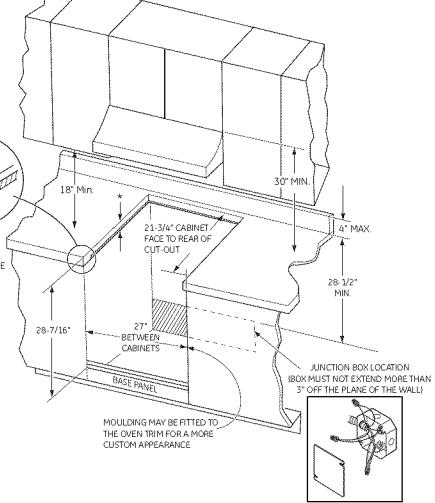
Allow 30" minimum clearance between surface units and bottom of unprotected wood or metal cabinet, or allow a 24" minimum when bottom of wood or metal cabinet is protected by no less than 1/4" thick flame retardant millboard covered with no less than No 28 MSG sheet metal, (.015"), .015" thick stainless steel, .024" aluminum or .020" copper.
