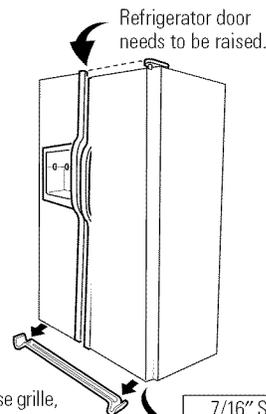
To remove the base grille, open the doors, remove the screw at each end of the base grille and then pull the grille straight out.
