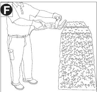
2. **WORKING POSITION** – Maintain proper footing and balance and do not overreach. Wear safety goggles, non-skid footwear and rubber gloves when trimming. Hold the tool firmly in both hands and turn the tool ON. Always hold the trimmer, as shown in **figure F**, with one hand on the switch handle and one hand on the bail handle. Never hold the tool by the blade guard.
