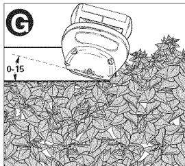
**CAUTION:** Do not use **model HT18** trimmer for cutting stems greater than 5/8 in. (16mm). Do not use **models HT20, HT22** trimmers for cutting stems greater than 3/4 in. (19mm). Use the trimmer only for cutting normal shrubbery found around houses and buildings.
