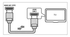
Using a High Speed HDMI cable, connect the HDMI OUT (ARC) connector on your SoundBar to the HDMI ARC connector on the TV.
