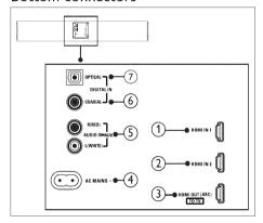
(1) HDMI IN 1 Connect to the HDMI output on a digital device.
