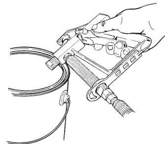
9. Trigger the gun and gradually turn the pressure control knob clockwise to 1/2 pressure. Continue to trigger the gun for approximately 30 seconds.
