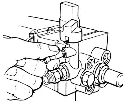
3. Press the return tube onto the brass fitting and fasten the return tube with the clamp provided.
