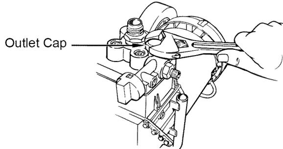
2. Leave the copper washer under the cap in place.
