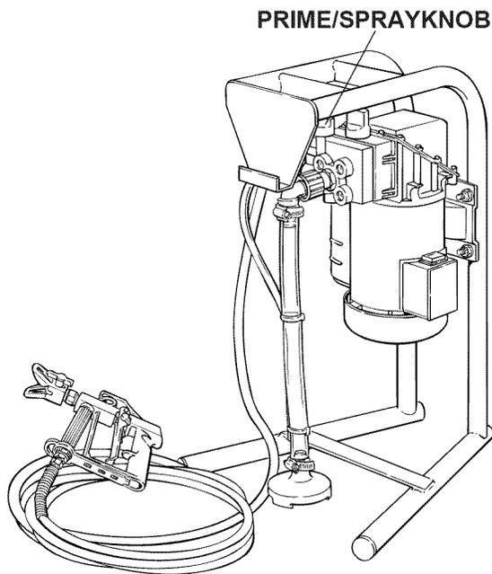
4. Turn the pressure control knob clockwise to its highest setting. The paint hose should stiffen as paint begins to flow through it.
