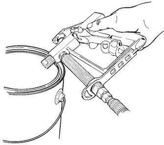
2. Turn the pressure control knob counterclockwise to the minimum pressure setting.
