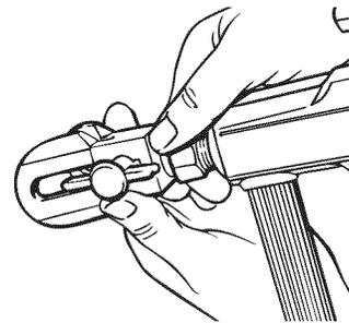
3. Unlock the trigger and squeeze it open, pointing the gun at a scrap piece of wood or cardboard. This allows pressure in the paint hose to blow out the obstruction. When the nozzle is clean, paint will come out in a straight, high pressure stream.
