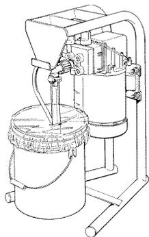
6. Wrap the spray gun assembly in a damp cloth and place it in a plastic bag. Seal the bag shut.
