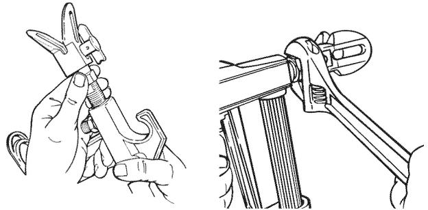
**NOTE: When attaching the tip to the gun, align the tip guard as shown in the figure below, then tighten with an adjustable wrench.**
