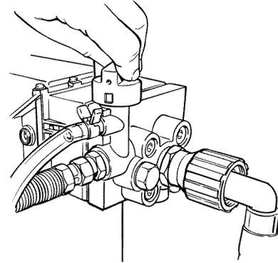
3. Trigger the gun to remove any pressure which may still be in the hose.
