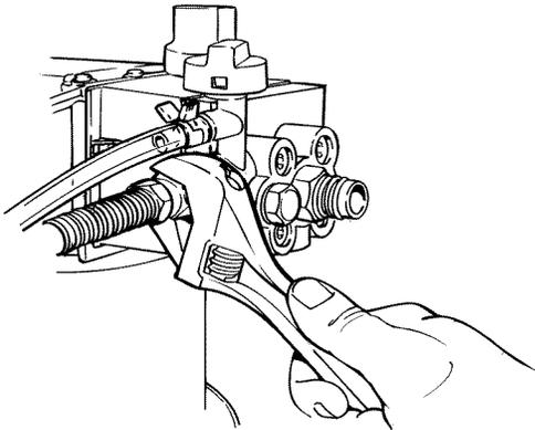
2. Attach the gun to the other end of the high pressure hose. Tighten securely with two adjustable wrenches.
