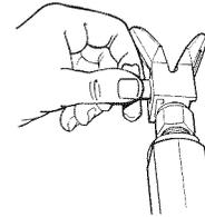
5. Attach the paint hose to the gun and tighten using two adjustable wrenches.
