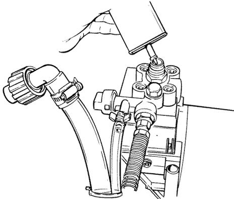
2. Make certain that the PRIME/SPRAY knob is set to PRIME (☉) and that the pressure control knob is turned counterclockwise to the lowest pressure setting.
