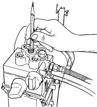
6. Put the palm of your hand over the inlet. Turn the pressure control knob clockwise to its maximum setting. You should feel suction coming from the inlet valve. If you do not, see the section on cleaning and servicing the outlet valve.
