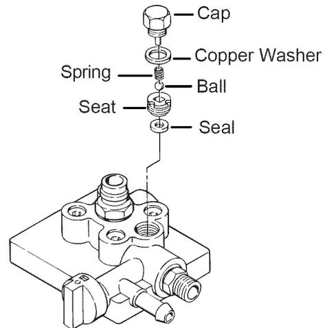
**NOTE: Wear on the ball is almost impossible to detect visually. To test for a worn outlet valve assembly, turn the pressure control knob clockwise to its highest setting and run water only through the sprayer for 10 to 15 minutes without triggering the gun.**
