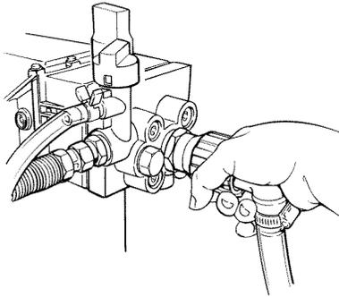
6. Unlock the gun and trigger it into the cleaning bucket until the hose is pumped dry.
