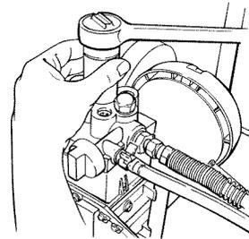
3. Test movement of the valve by pushing on it from the open end of the valve housing with a screwdriver or the eraser end of a pencil. It should move about 1/16 of an inch. If it does not move, it should be cleaned or replaced.
