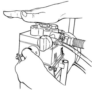
7. Turn the pressure control knob counterclockwise to the minimum pressure setting.
