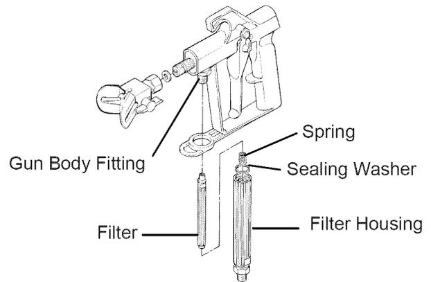
9. Replace the spring and sealing washer into the base of the filter housing.
