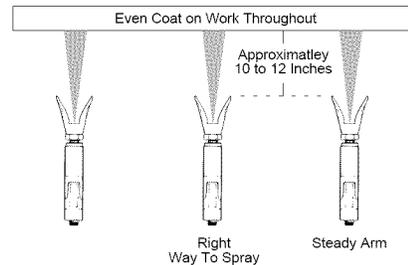
Keep the spray gun perpendicular to the surface, otherwise one end of the pattern will be thicker than the other.
