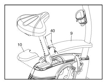
Next, locate the Reed Switch (21). Loosen, but do not remove, the M4 x 16mm Screw (40).
