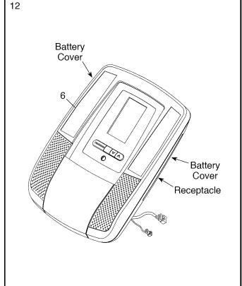
13. While a second person holds the Console (6) near the Console Plate (19), connect the wires on the Console to the Main Wire (31) and to the Pulse Wire (52).
