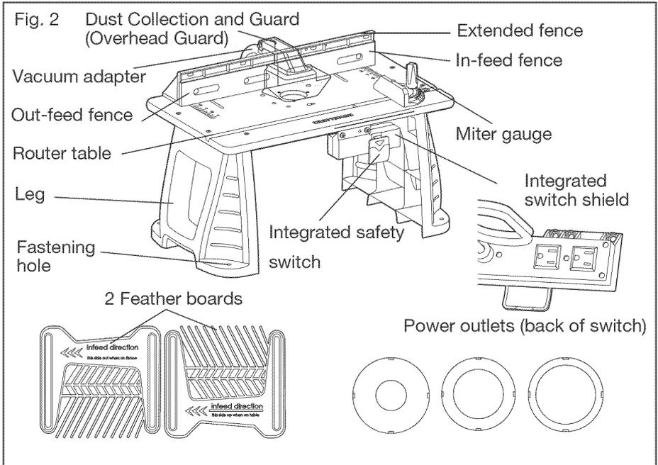
Your router table has a precision-built electric switch box and it should be connected to only a 120-volt, 60-HZ AC power supply (normal household current). DO NOT operate on direct current (DC). The large voltage drop would cause a loss of power and the motor would overheat. If the router table does not operate when plugged into correct 120-volt, 60-HZ AC ONLY outlet, check the power supply. The router table comes with a 6-ft. power cord (no adapter needed).
