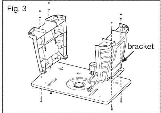
4. Place small plain washers (14) onto each of two short pan-head screws (13). Insert the short pan-head screws up through the holes in the table and through the holes in the leg bracket. Place a small plain washer (14), a spring washer (15), and nut (16) on the threads of the screw (13). Loosely tighten the nuts (Fig. 3).
