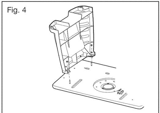
5. Place a small plain washer (14) onto each of two long pan-head screws (12). Insert the long pan-head screws up through the other two holes in the tabletop and through the corresponding holes in the leg. Place a small plain washer (14), a spring washer (15), and nut (16) on the threads of the screw (12) as shown in Fig. 4.
