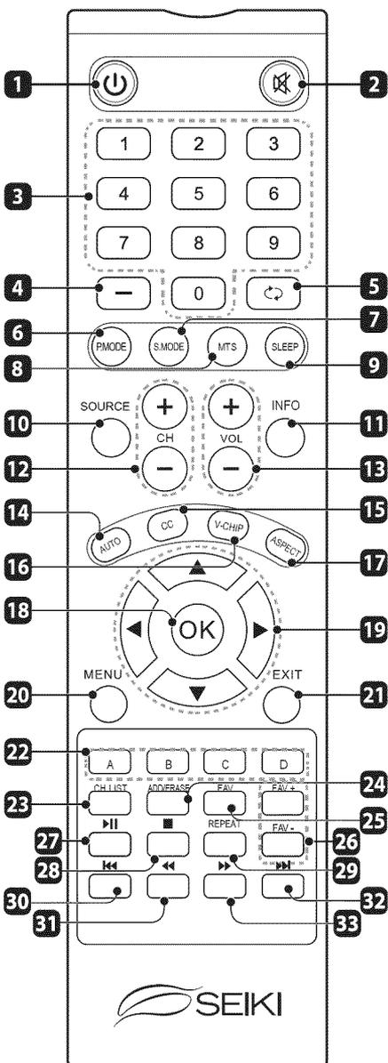
1. **⏻**: Switch the TV between on and standby mode.
