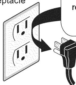
Power supply cord with 3-prong grounding plug
