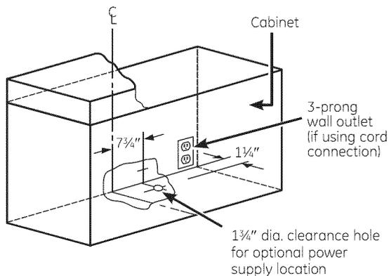
**NOTE:** If using optional Power Cord Kit JXHC1, feed the power cord through the hole in the top cabinet while raising the hood. Loop any excess length of cord and tie away with a suitable tape or tie.
