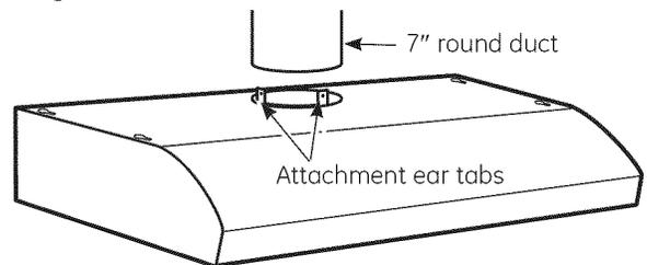
Use duct tape to make joints secure and airtight.
