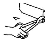
\* **IMPORTANT:** If a rectangular-to-round transition adaptor is used, the bottom corners of the damper will have to be cut to fit, using the tin snips, in order to allow free movement of the damper. Equivalent lengths of duct pieces are based on actual tests and reflect requirements for good venting performance with any hood.
