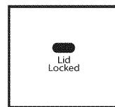
If you need to open the lid, press START/Pause. The lid will unlock once the washer movement has stopped. This may take several minutes if the load was spinning at high speed. Press START/Pause again to resume the cycle. Avoid opening the lid during sensing. The sensing process will start over when the washer is restarted.
