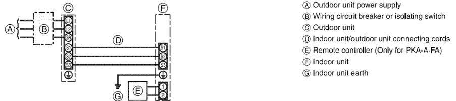
\* Affix a label A that is included with the manuals near each wiring diagram for the indoor and outdoor units.
