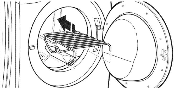
2. Align the two hooks on the front of the drying rack with the holes in the dryer door opening and press down fully into holes. Rest the rear support on the dryer back ledge.
