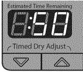
When you select a Manual Cycle, the default time appears in the display. Use the ▲ and ▼ buttons to increase or decrease the time in 1 minute increments. Press and hold to change the time in 5 minute increments.
