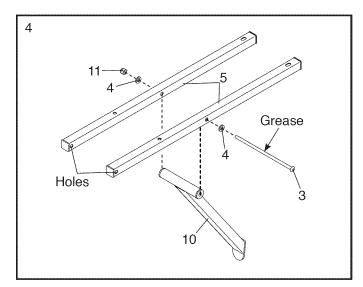
5. Apply a small amount of the included grease to an M10 x 202mm Bolt (3).
